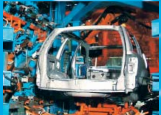
Body and assembly: Force and position control of weld tips, material clamping, locating, and conveying
