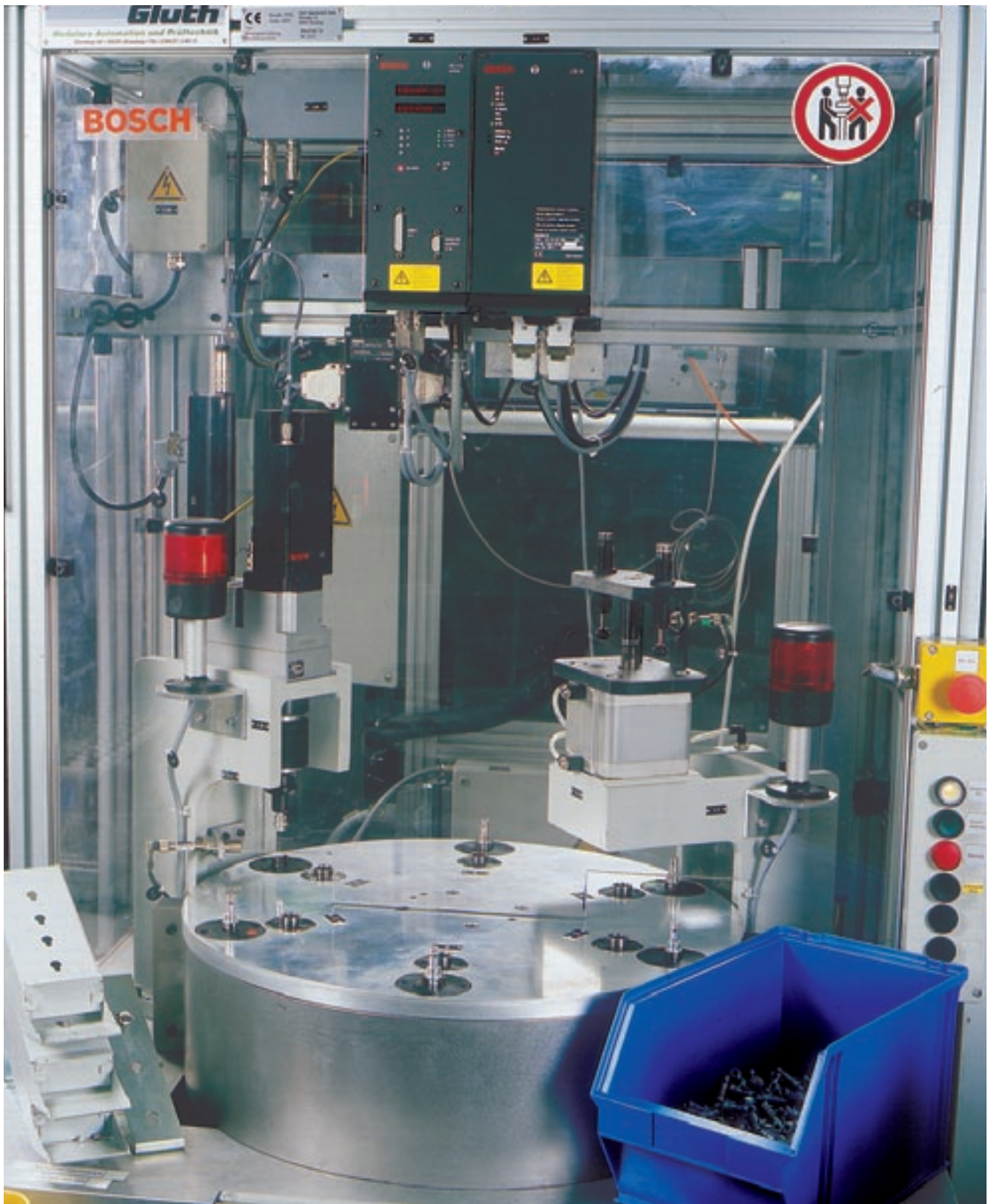
Press-fit station in injection-pump production
