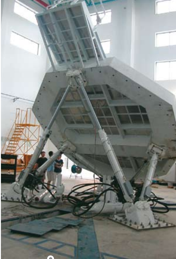
Hydraulic motion system with Rexroth servo valve STWS0034-10 and customer supplied platform, for full flight simulation
